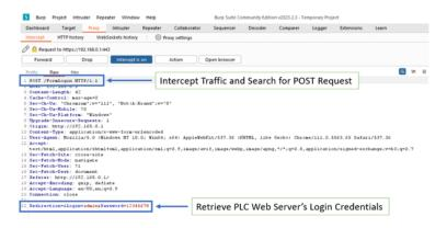
3. The hacker views the login credentials displayed in Burp Proxy, showing encryption between the browser and PLC before sending the login credentials.
